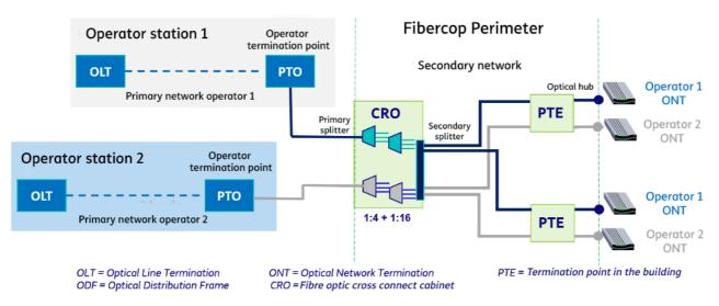
In the case of the towns with FTTH already developed before the establishment of FiberCop (infrastructures developed by the company Flash Fiber, whose ownership was purchased by FiberCop), the reference architecture of the Semi-GPON network envisages a splitting distributed along the secondary network (thus not concentrated inside the CRO, as seen above); the first level of splitting occurs at the CNO (Optic Node Centre) and a second level at the PTE, for an overall ratio still equal to 1:64.
