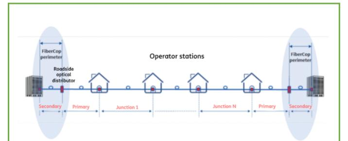
In the event of available space, the first PTO will generally be positioned directly inside the manhole in the road, in the vicinity of the Optic Node Centre (CNO) or of the Fibre Optic Cross Connect Cabinet (CRO) of the FiberCop FTTH network. In the absence of space available in the network infrastructures already prepared (CNO/CRO), the Operator's Termination Point (PTO) must be created for the purpose, according to the instructions that FiberCop will provide in the specific cases.
